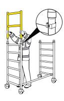
Fit a diagonal brace between the 5th rung of the base unit and the lower rung of a guardrail frame.
