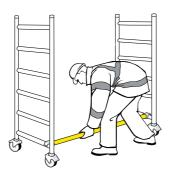
Fit the four spring interlock clips supplied with the guardrail pack. Expand the clips over the top of the base unit uprights and then slide down to engage the pin on the clip into hole in the upright.
